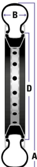
**ETRTO:** The standard definition of the "European Tyre and Rim Technical Organisation" is: section width **B** and seat stay diameter **D** in millimetres. **French:** Outer diameter **A** x width **B** in millimetres. **English:** Outer diameter **A** x width **B** in inches.
