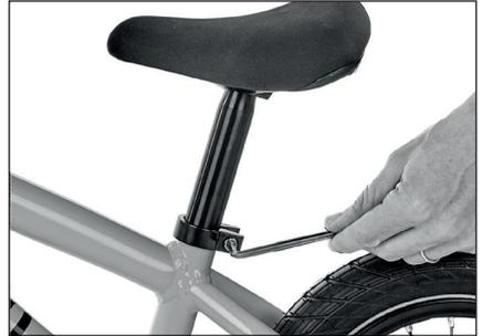
3. Tighten the saddle clamp bolts to a torque of 5 Nm.
