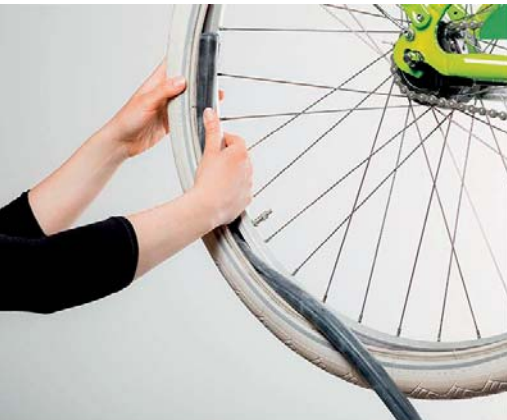
Step 9 of 14: Insert the GAADI inner tube with the short end first.
