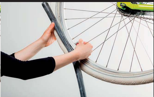
Step 8 of 14: Screw the valve cap onto the valve slightly. Do not tighten it yet.
