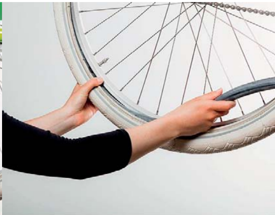
Step 10 of 14: Insert the long end of the GAADI inner tube.
