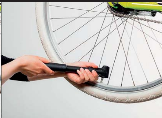
Step 14 of 14: Inflate the tyre and check that the tyre's bead is seated evenly on the rim.
