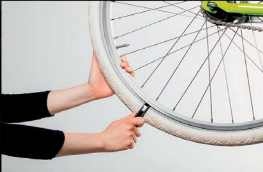
Step 1 of 14: Use a tyre-lever to lift the tyre's bead over the rim.
