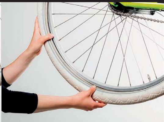
Step 12 of 14: Insert the tyre's bead back into the rim.
