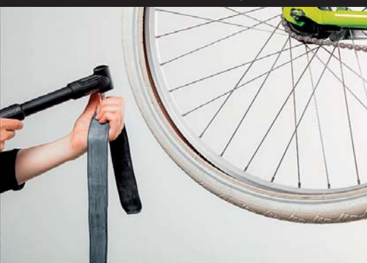
Step 5 of 14: Inflate the GAADI inner tube slightly before inserting it. This facilitates the assembly and avoids that the inner tube gets twisted.
