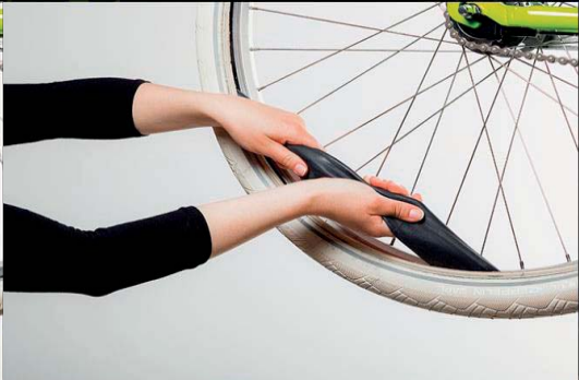
Step 2 of 14: Pull out the old inner tube.
