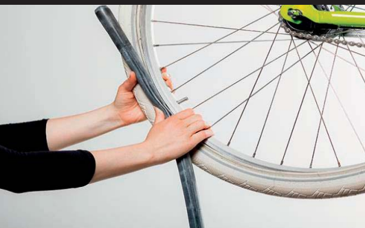
Step 7 of 14: Push the valve through the valve hole of the rim.
