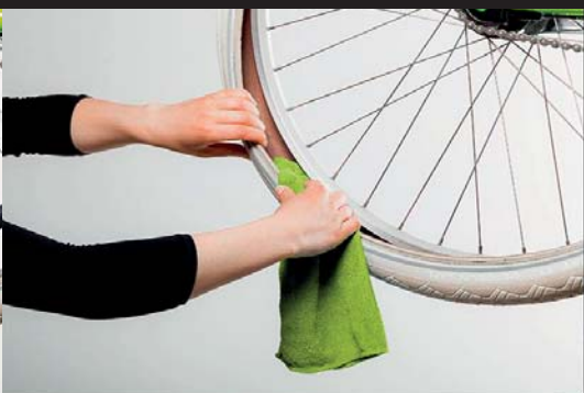
Step 4 of 14: Check the tyre's inside carefully and remove glass etc.
