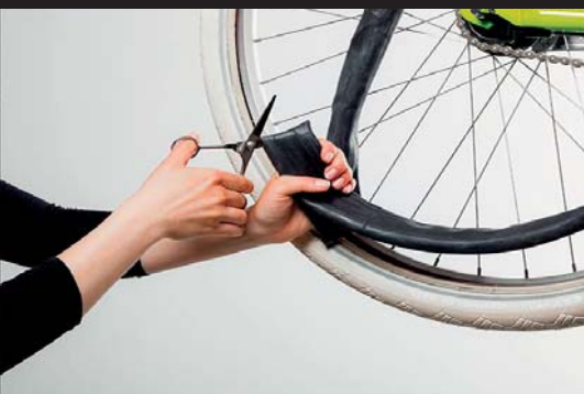
Step 3 of 14: Cut the old inner tube in half. This should be done with small scissors as it is the safest way to do so.
