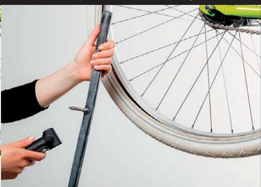
Step 6 of 14: Inflate the GAADI inner tube slightly before inserting it. This facilitates the assembly and avoids that the inner tube gets twisted.
