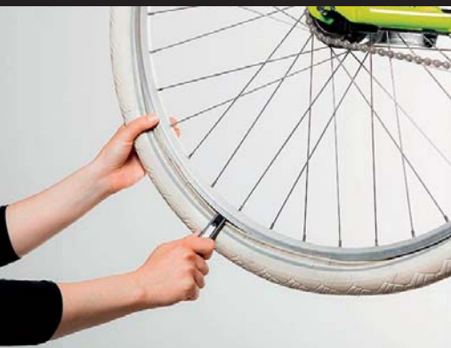
Step 13 of 14: Use the tyre-lever again to facilitate inserting the last bit of the bead.
