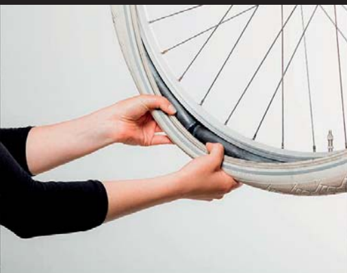
Step 11 of 14: Both ends of the GAADI inner tube should be joined together.
